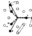
TAIL & PILOT LTS ON (TURN LT SW RIGHT TO P) IGNITION ON (TURN IGNITION KEY RIGHT)
